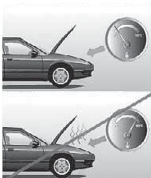
Spark plug installation and removing from the cylinder head must be carried out only when the engine has ambient temperature. Removing and installing spark plug while hot can actually cause thread and cylinder head damage.
