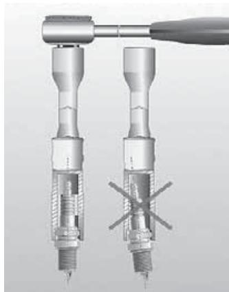
Use always the proper spark plug wrench which is not too loose and is provided with centring ring from soft material.
