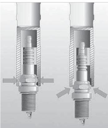
Tightening torque can be applied in such case only when the wrench is put on across the whole length of hexagon of spark plug metal shell.
